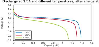
Discharge at 1.5A and different temperatures, after charge at C
